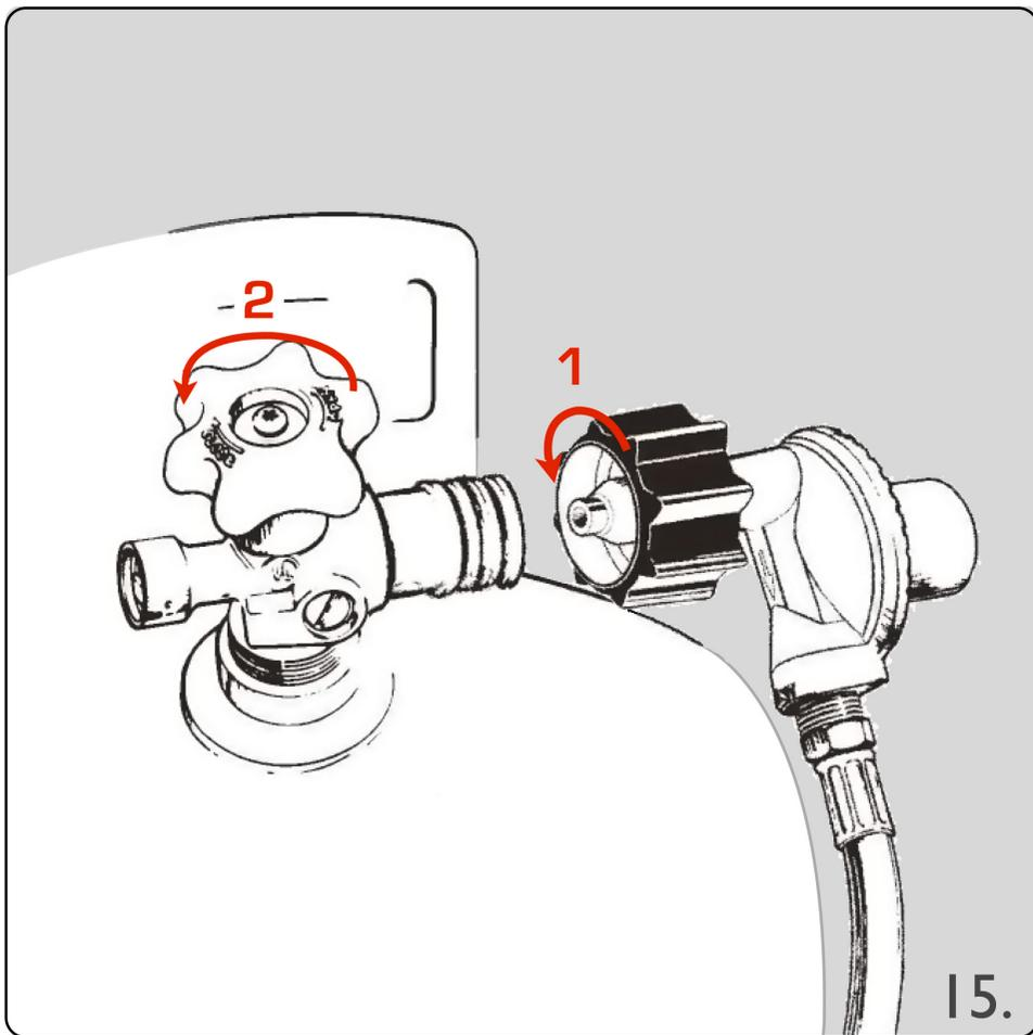
15. Attach the regulator to the propane tank. Open the valve on the propane tank.
