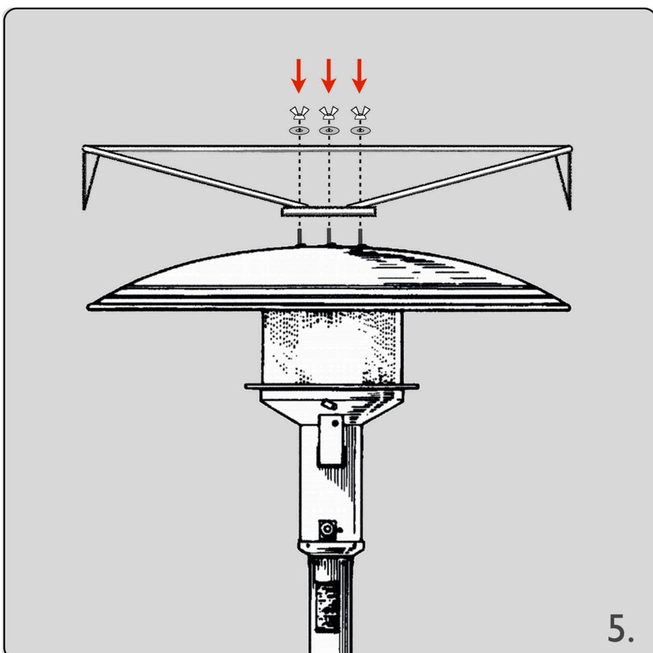
5. Attach the reflector and shade bracket to the bolts on top of the heater head with wing nuts and washers.
