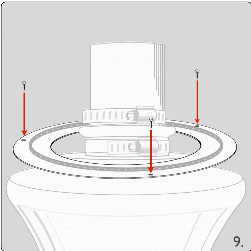
9. Attach optional light ring to the base of the Kindle neck using the 3 small self-tapping screws. Be careful not to over-tighten.
