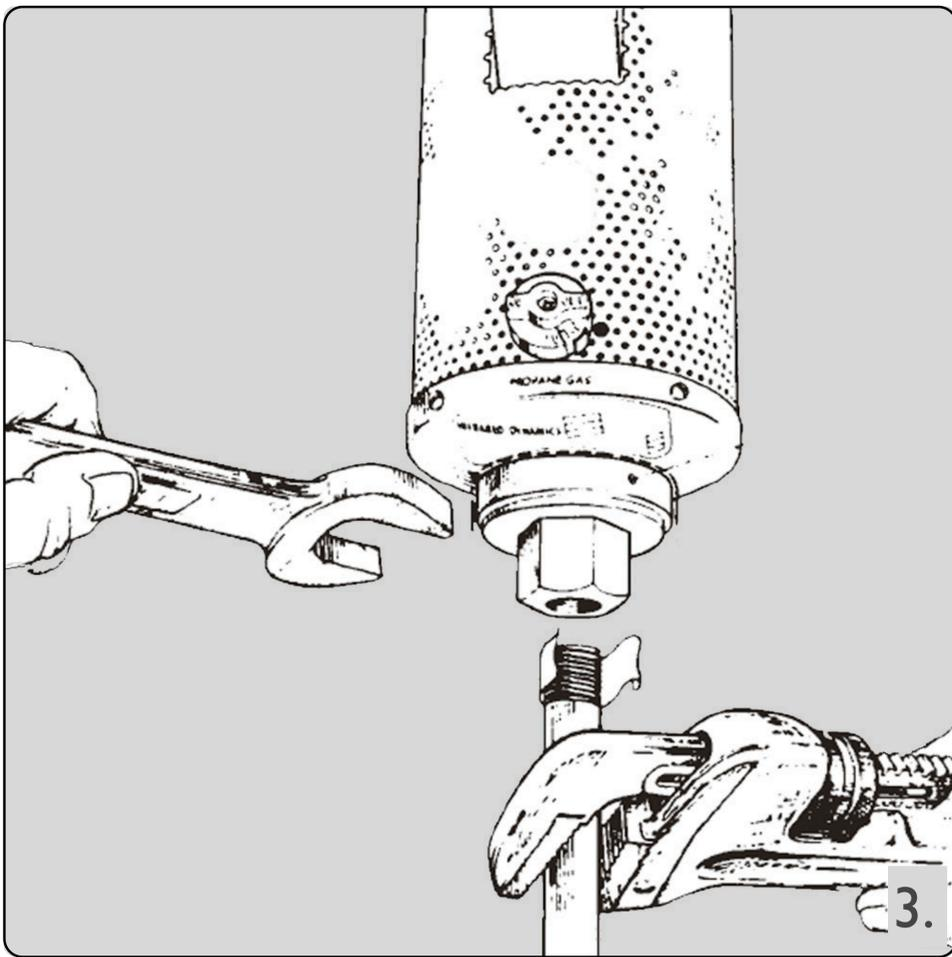
3. Using two wrenches, firmly attach the end of the gas pipe that has the teflon tape to the heater head.
