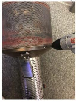
Adjust electrode so that it is about 1/4" from pilot shield. A small spark should be seen when pressing red ignitor button.
