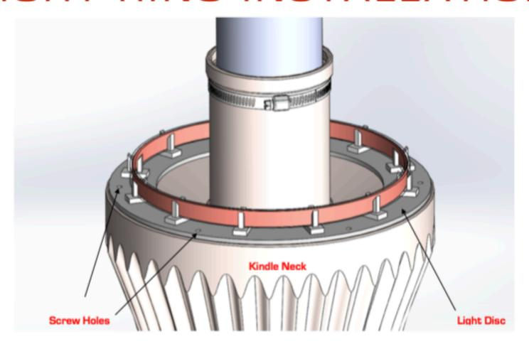
• Line up the edge of the light disc with the edge of the Kindle neck's base. Alternating holes, screw the three provided screws into the Kindle neck's base. *Note: there are no screw holes; the screws go directly into the material of the Kindle neck.* Please be careful not to over tighten screws or you risk damaging the light ring.
